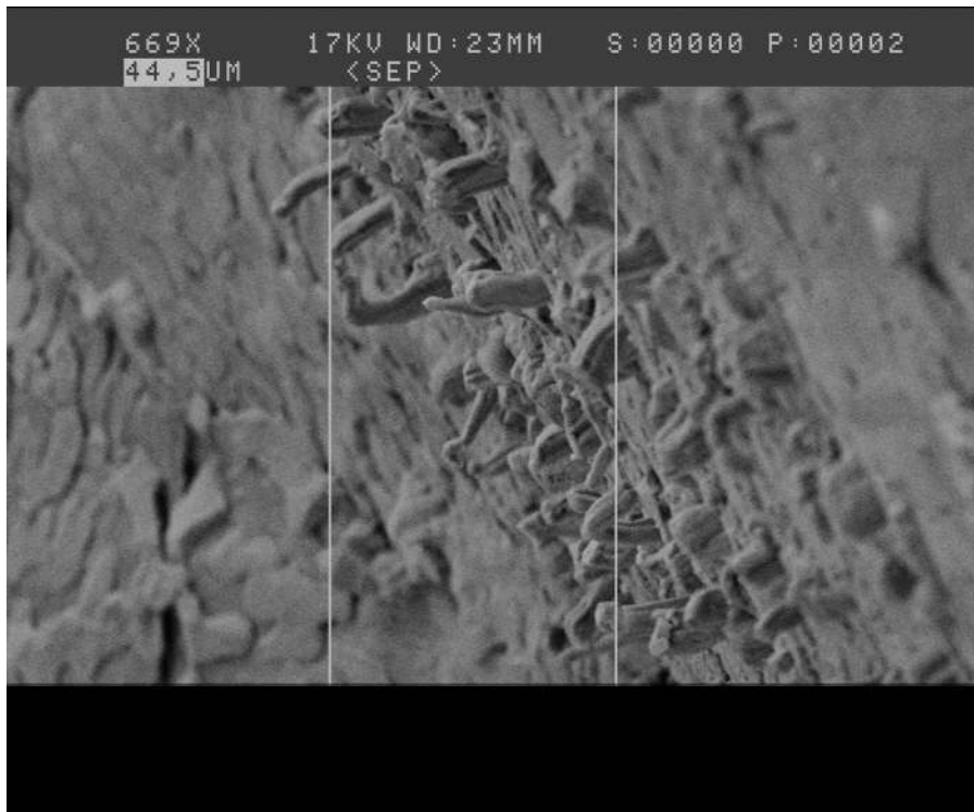
IMAGE 1 – Whisker Growth on Capacitor End-Terminations
