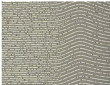
FIGURE 2. Undulating electrode and dielectric layers.
