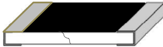
FIGURE B-12. Substrate crack.
