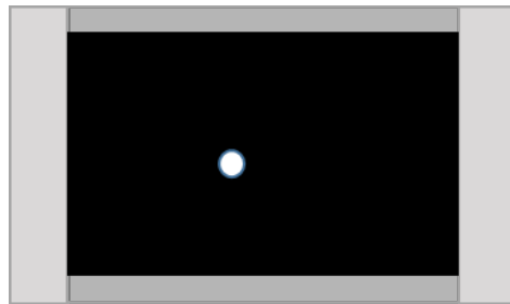
FIGURE B-13. Metal particle on the passivation.
