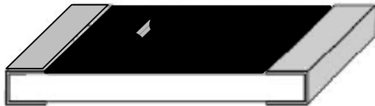
FIGURE B-14. Top coat exposing underlying resistor element.
