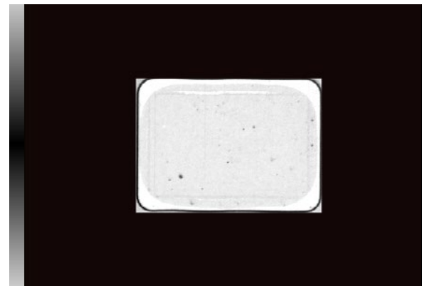
Example 2030-2f: Lid to TIM reflection mode image through lid to the thermal interface material.
