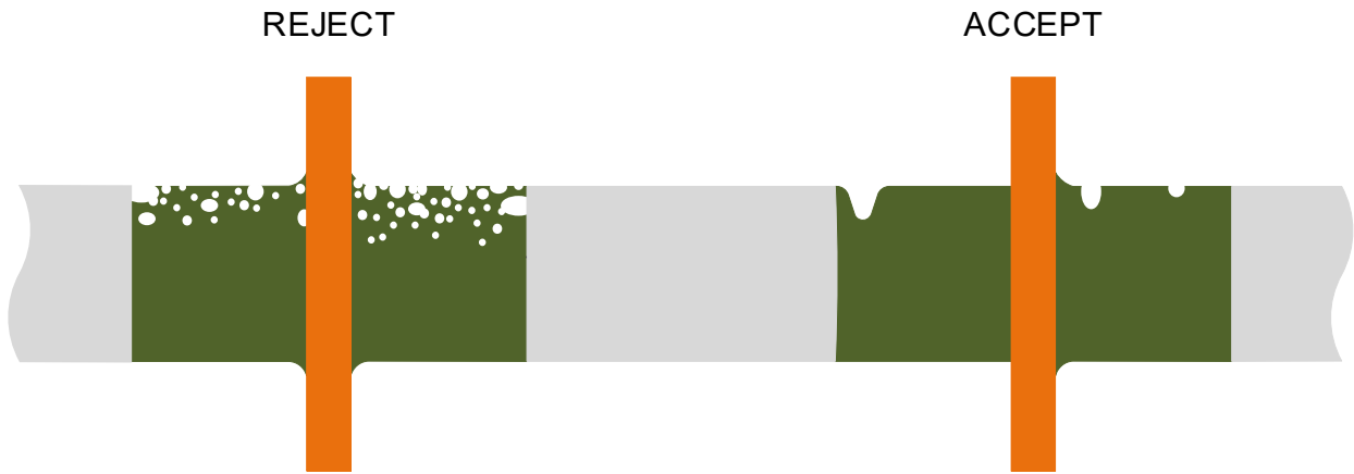
FIGURE 2071-4. Open surface bubble(s) in the glass seal surface.
