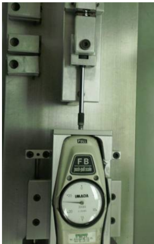
FIGURE 2038-1. Sample apparatus fixture with force measuring gauge.
